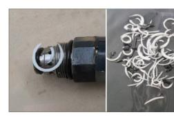
PTFE back-ups are pinched and broken during installation; leading to seal failure.
