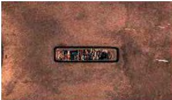
Figure 2: Pin on Flat Wear Test Results for Alloy 718 Coated with TriCom and Tribaloy T-800.
