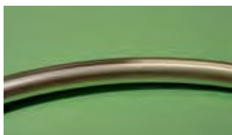
Figure 2: Parker Hannifin's Silver-Indium diffused plating
