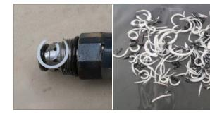
PTFE back-ups are pinched and broken during installation; leading to seal failure.
